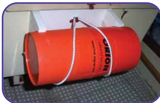
The finished mount installed below the companionway for quick access.
