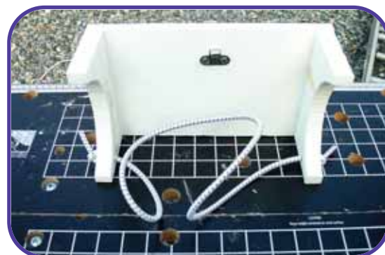
Overall view of the mount ready to install. Note the bungee cord and the hammock hook.
