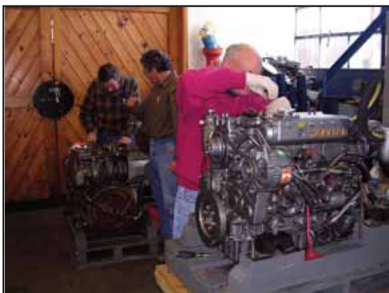
Students starting valve adjustments on two of the six-cylinder Yanmars.
