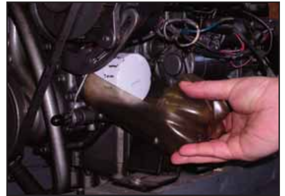
One of the more high tech tools ( a 1 liter soda bottle) for changing oil filters without pouring oil into the bilge.
