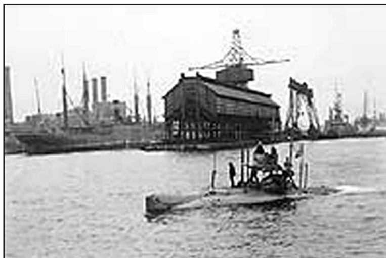
USS Plunger , a 107-ton Holland-type submarine built at Elizabethport, NJ, was commissioned in September 1903.
