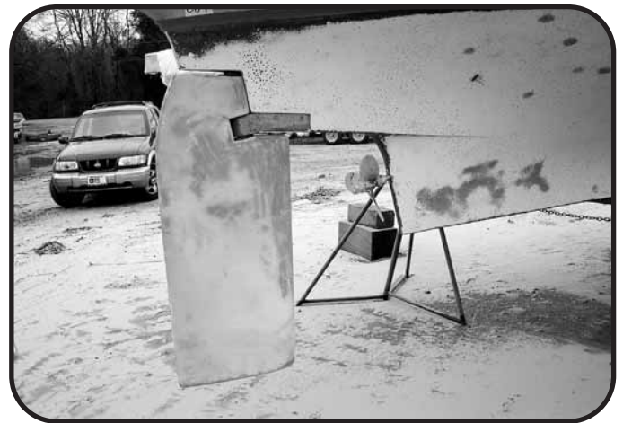
The opposite side, several minutes work with a sandblaster.
