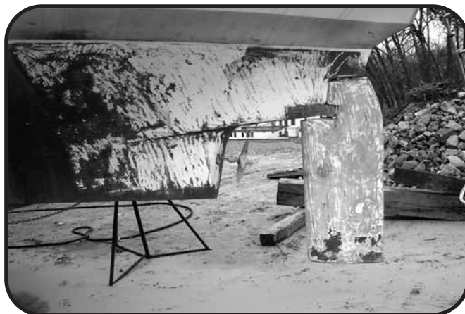
A weeks worth of work with paint stripper and scrapers.
