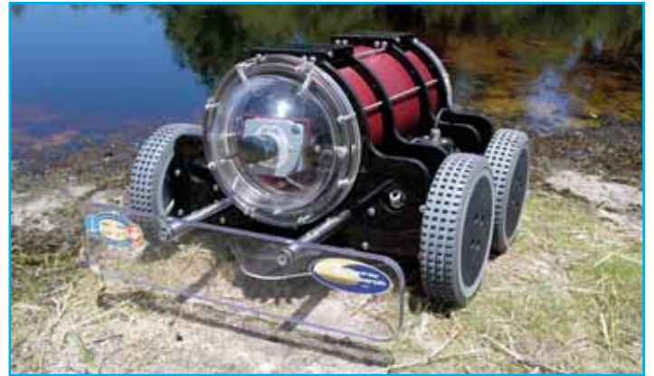
The Hull Bug attaches to the hull of a vessel while still in the water and roams the surface of the hull looking for barnacles and marine growth to remove.
