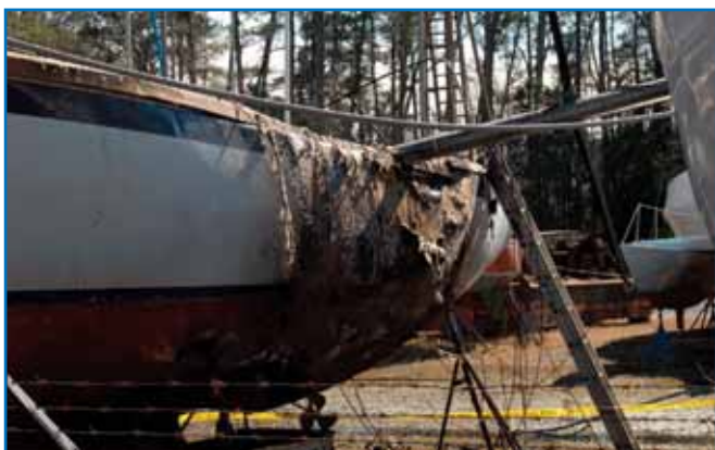
A fuel tank leak and electricity combined to destroy this sailboat on the hard.
