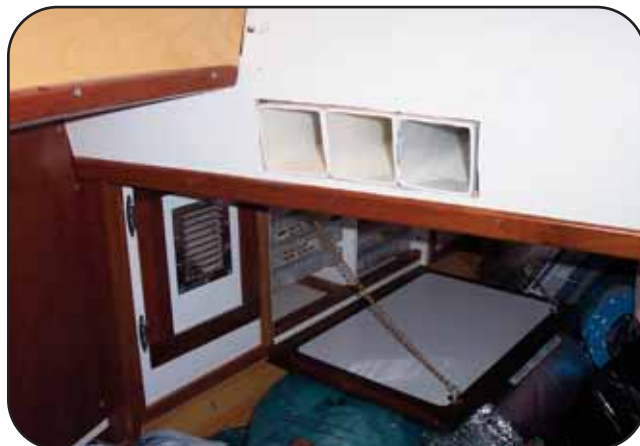
Tube opening cut, tubes cut to length and in place
